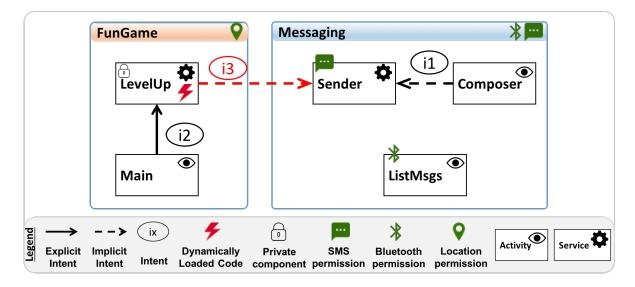
Figure 1: Component-based architecture of a vulnerable Android system.
